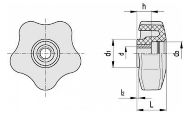
$\begin{array}{lll} D & = 40 \\ d1 & = 17 \\ d3 & = 12.5 \\ dh & = 8 \\ h & = 10 \\ I2 & = 1 \\ L & = 17 \\ Weight in (g) = 10 \\ \end{array}$
